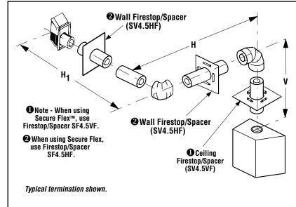
See Table 8 on Page 20 as an aid in venting component selection for a particular range of exterior wall thicknesses.
